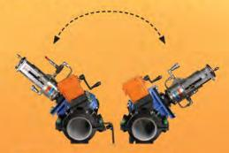
While maintaining system line pressure, mill a slot over a 120° path
